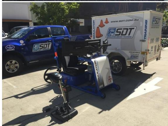
**Frame:** Metal and Plastic construction with height adjustable steering column
